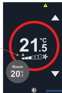
The system uses the last command principle. If the fan speed has been set/changed from the network then the display goes to automatic mode (showing 'A' next to the line bar if Auto option selected). When the device is manually overridden then the 'A' symbol changes to 'M' indicating manual operation (only if Auto option has been selected for Manual Control). Otherwise the screen shows only the selected Fan Speed.
